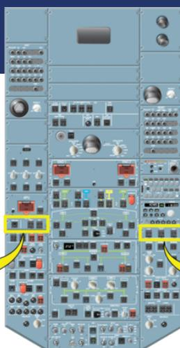
Example of pushbutton-switches on the overhead panel of an A330 aircraft
