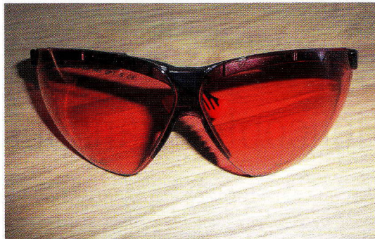
Fig. 3: The Laser-2000 XC goggles proved to be the most appropriate ones for LASER protection (Photograph: M. Vandenavenne)
