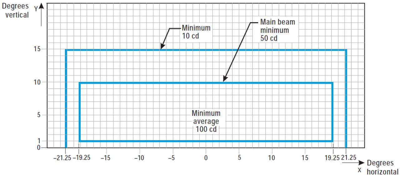
Figure U-18. Isocandela diagram for taxiway centre line (7.5 m spacing) and stop bar lights in curved sections intended for use in runway visual range conditions of less than a value of 350 m
