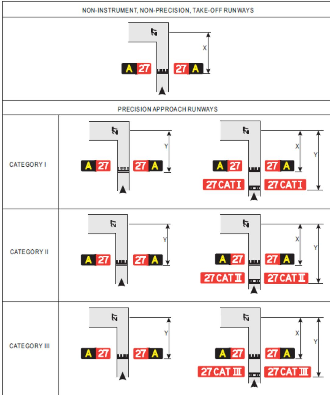
Note. – Distance X is established in accordance with Table D-2. Distance Y is established at the edge of ILS/MLS critical/sensitive area
