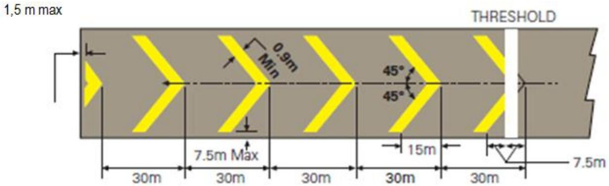
Figure R-2. Pre-threshold area marking
