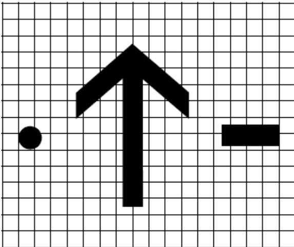
Note 1. — The arrow stroke width, diameter of the dot, and both width and length of the dash should be proportioned to the character stroke widths.
