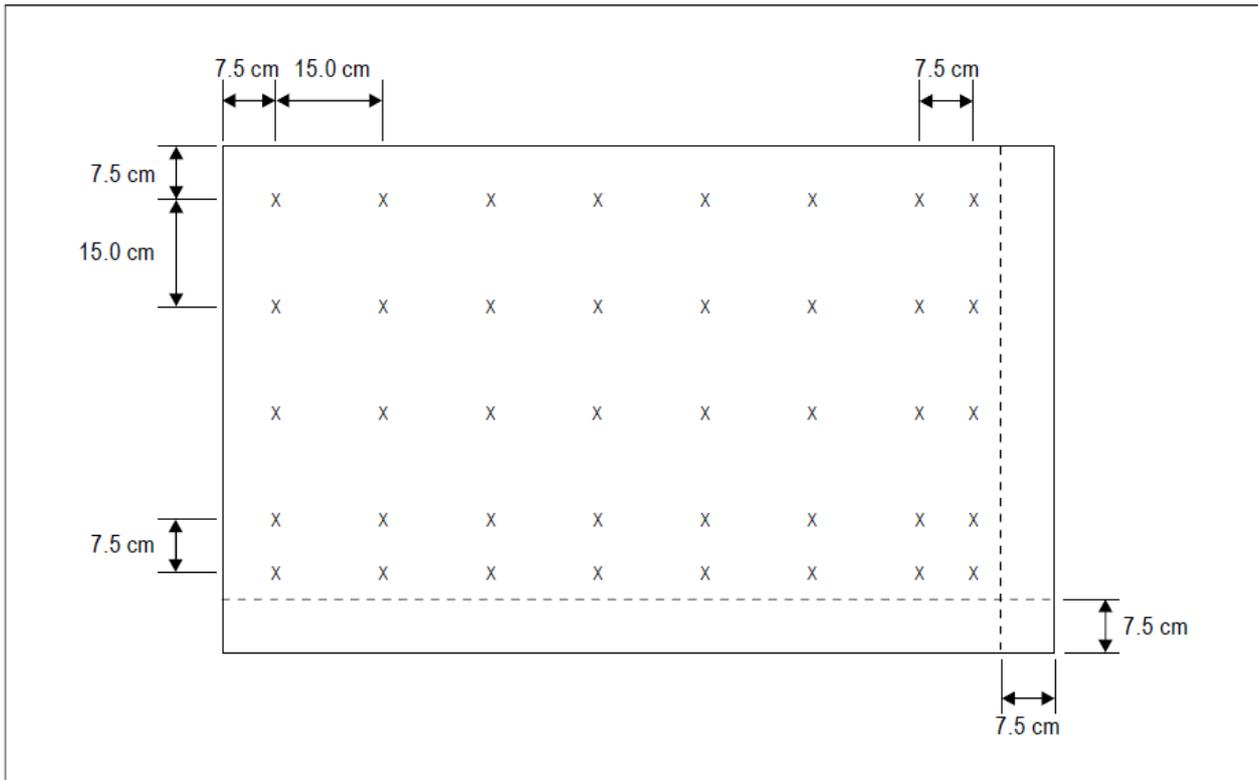
Note 1.— The average luminance of a sign is calculated by establishing grid points on a sign face showing typical inscriptions and a background of the appropriate colour (red for mandatory instruction signs and yellow for direction and destination signs) as follows:
