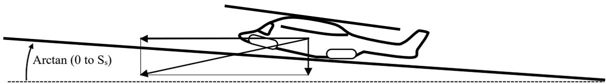
b) Water entry into inclined plane of stationary water, steepness range - zero to significant steepness ( $S_s$ )
