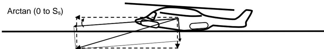
c) Water entry into a stationary horizontal water surface using an equivalent water entry angle and velocity relative to the water surface (Dashed arrows show required horizontal and vertical speeds)
