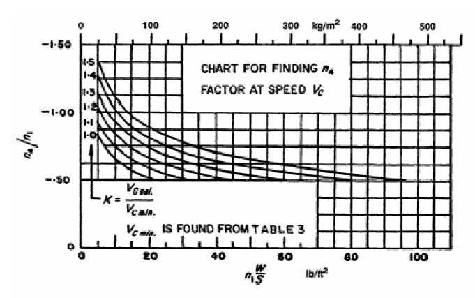
FIGURE A2 CHART FOR FINDING n4 FACTOR AT SPEED  $V_{\text{C}}$ .
