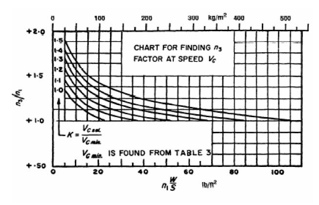
FIGURE A I CHART FOR FINDING n3 FACTOR AT SPEED  $V_{\rm C}.$
