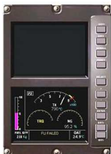
Here illustrated on AS 350 B3 and EC 130 B4, when upper screen fails, the FLI fails to.
