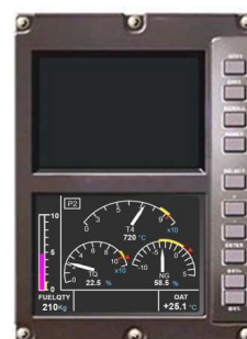
On AS 350 Series and on EC 130T2, when upper screen is failed, FLI fails but the 3 parameters (TOT, Tq & NG/Delta NG) still displayed on the lower screen.
