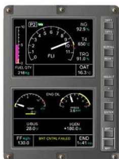
Here illustrated on AS 350 B3 and EC 130 B4, when upper screen fails, the FLI fails to.
