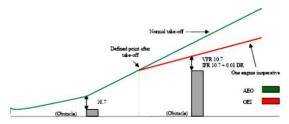
Figure 4: Performance Class 2 Obstacle Clearance (plan view)
