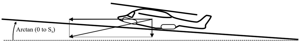
b) Water entry into inclined plane of stationary water,
