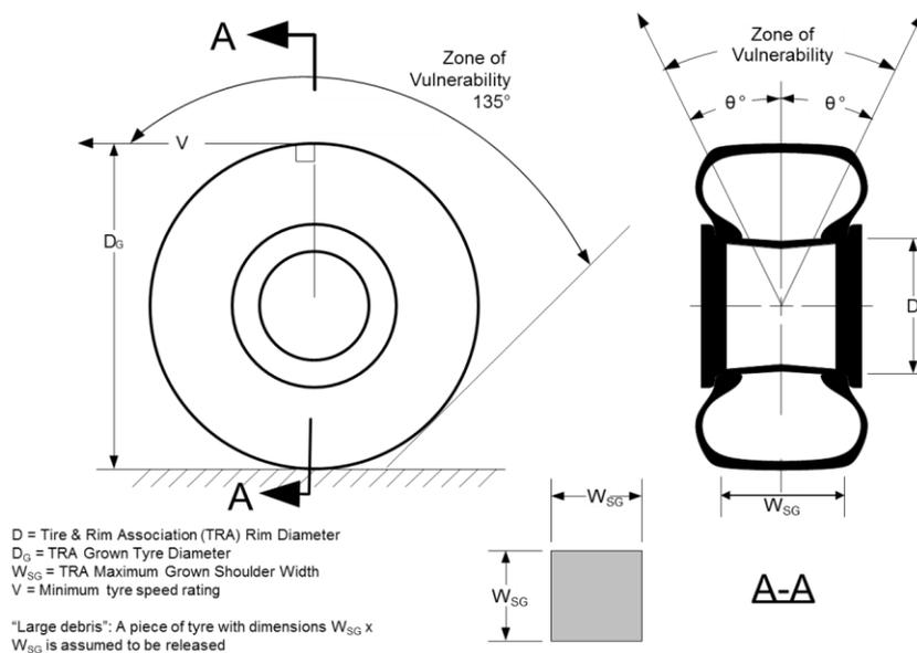
**CS-25 BOOK 2**(2) Protection of the fuel tank structure and pass-fail criteria on effects of penetration
