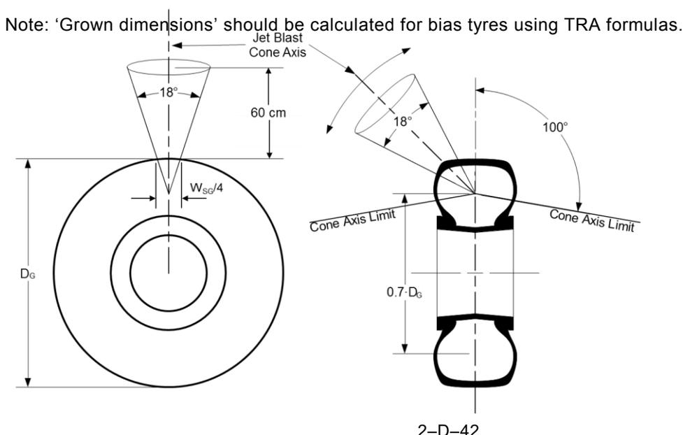
Figure 4b – Tyre Burst Pressure Effect – Bias Tyre
