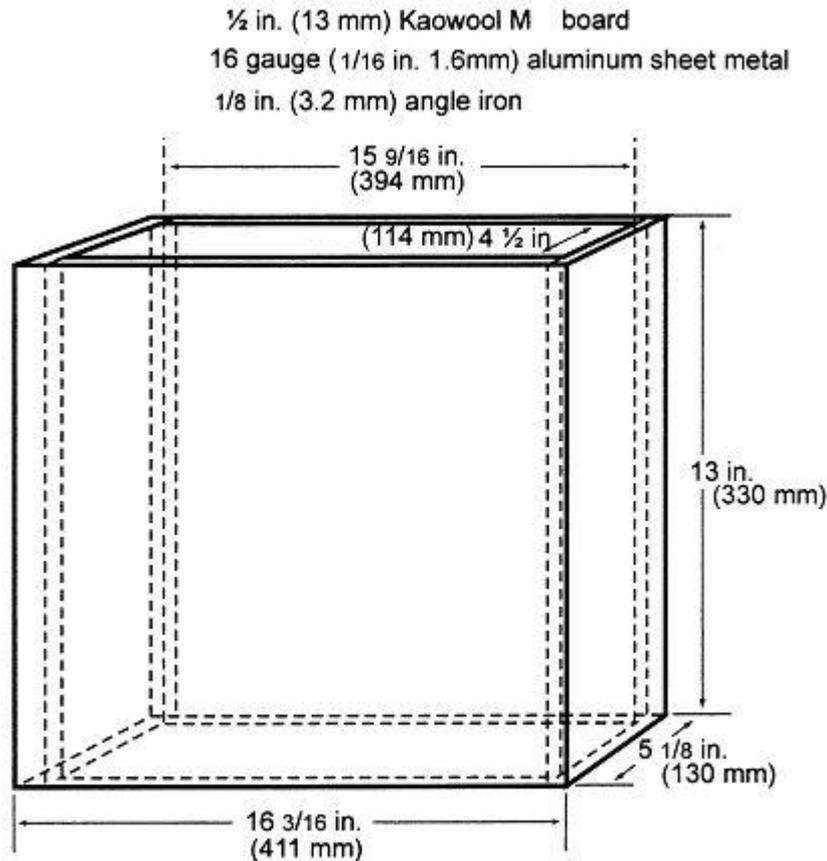
Figure 2 - Internal Chimney
