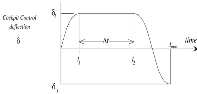
**CS 25.333 Flight manoeuvring envelope**
