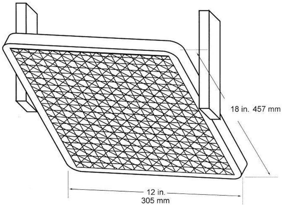
Figure 3b – Air Propane Radiant Panel
