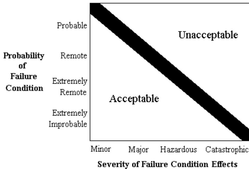
b. The classification of the Failure Conditions associated with the severity of their effects are described in Figure 2a.
