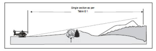
a) Approach and take-off climb surfaces - 4A\* slope profile - 4.5% design
