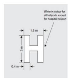
Figure F-3. Heliport identification marking
