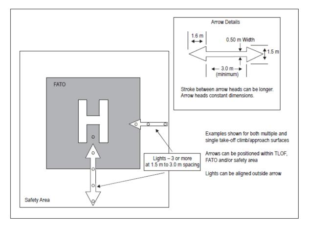
Figure GM1-F-2. Flight path alignment guidance markings and lights
