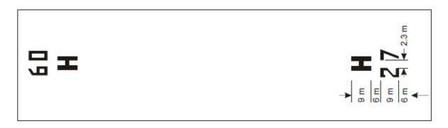
Figure F-2. FATO designation marking and heliport identification marking for a runway-type FATO
