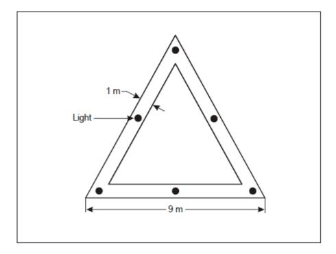
Figure F-9. Aiming point marking and lighting
