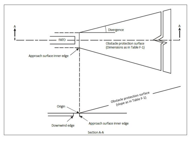
Figure F-7. Obstacle protection surface for visual approach slope indicator systems
