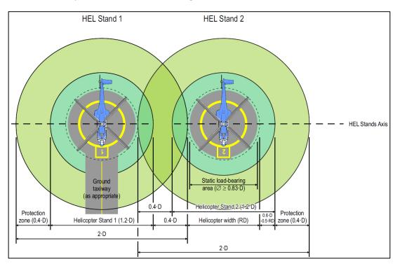
Figure GM D-1. Reduced separation distance between helicopter stands
