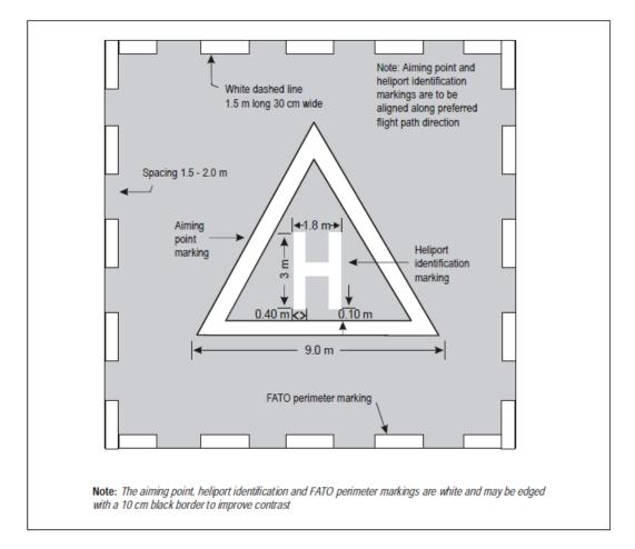
Figure F-1. Combined heliport identification, aiming point and FATO perimeter marking
