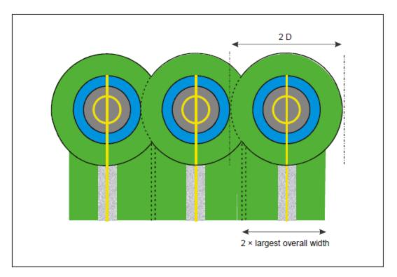
Figure D-3. Helicopter stands designed for hover turns with air taxi-routes/taxiways — non-simultaneous operations
