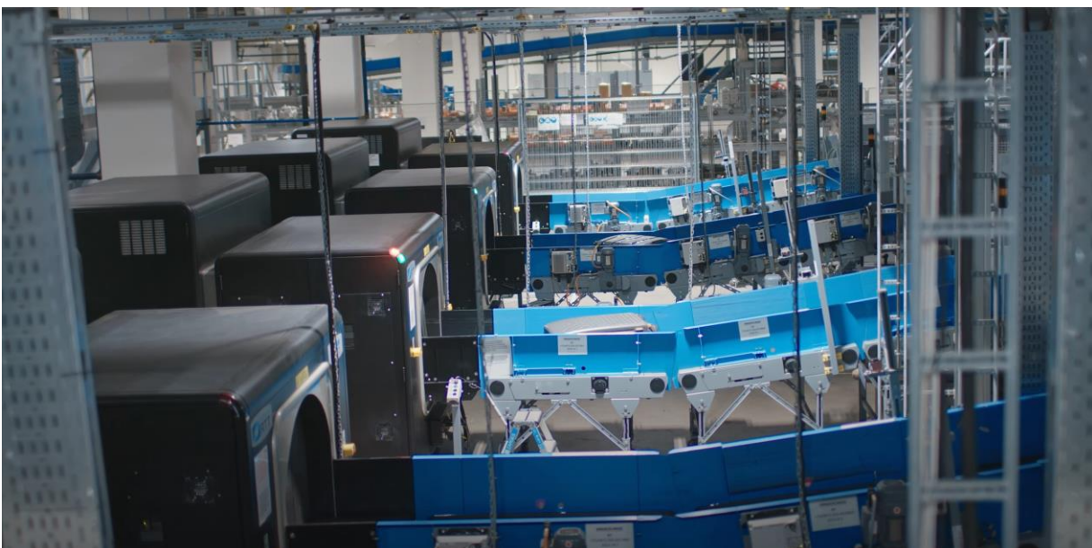
Image 1 - shows a baggage handling system conveying passenger baggage through four Rapiscan EDS machines, screening for explosives.
