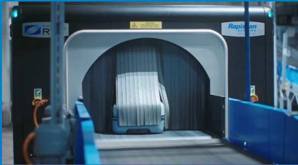
Image 2 – shows a bag going through the EDS machine.
