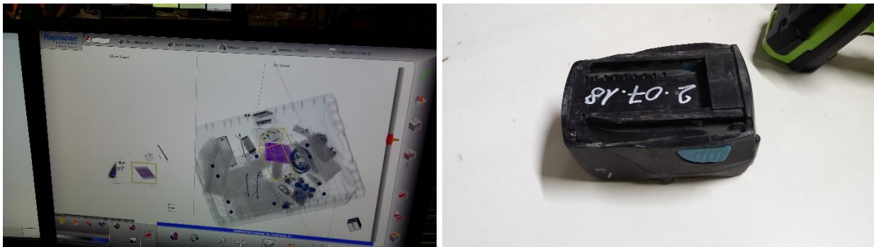
Image 6 – shows Rapiscan screener GUI highlighting a lithium battery alarm image and the actual item found (power tool battery).
