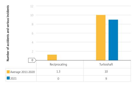
• Figure 65 Accidents and serious incidents by propulsion type involving commercial air transport helicopters
