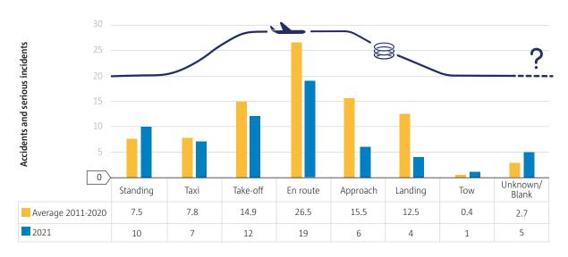
Figure 9 Accidents and serious incidents by phase of flight involving commercial air transport airline and air-taxi aeroplanes
