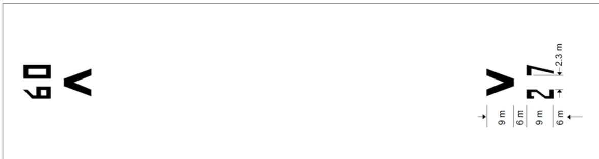
**Figure E-3.** FATO designation marking and vertiport identification marking for a runway-type FATO
