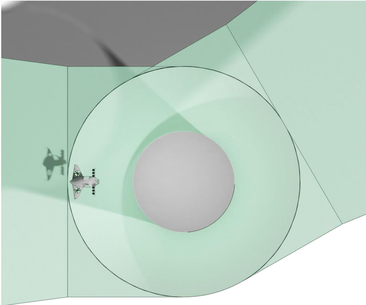
**Figure D-18.** Vertiport omnidirectional obstacle-free volume with discrete planar approach and take-off climb surfaces — top view
