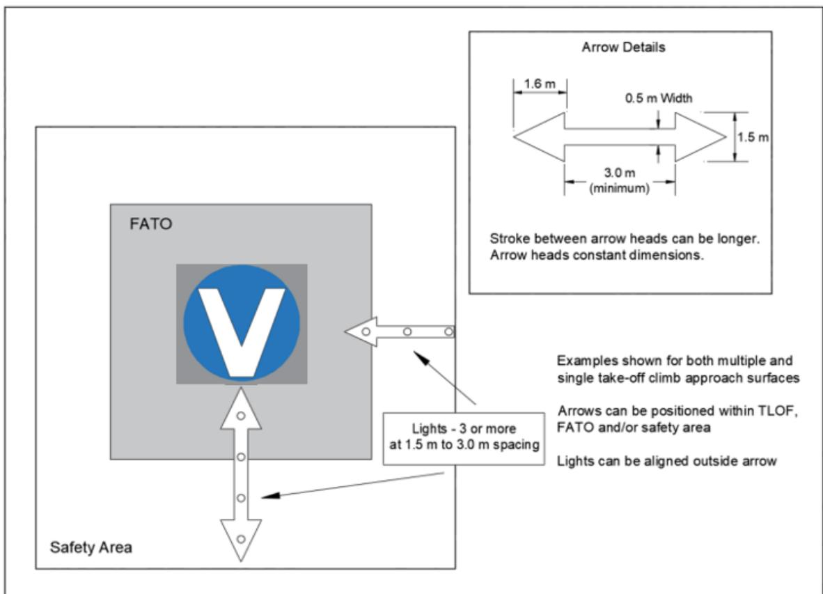
Figure E-14. Flight path alignment guidance markings and lights
