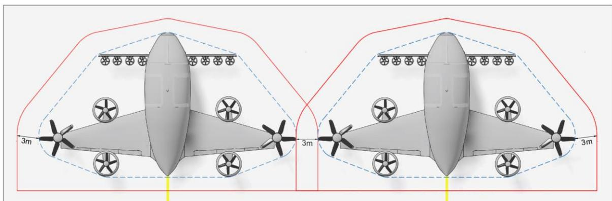
**Figure C-8.** VTOL-capable aircraft stands with a protection area
