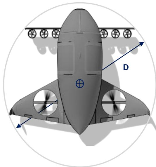
**Figure D-23.** Dimension 'D' and centre of the smallest enclosing circle
