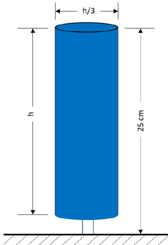
**Figure E-10.** VTOL-capable aircraft taxiway edge marker
