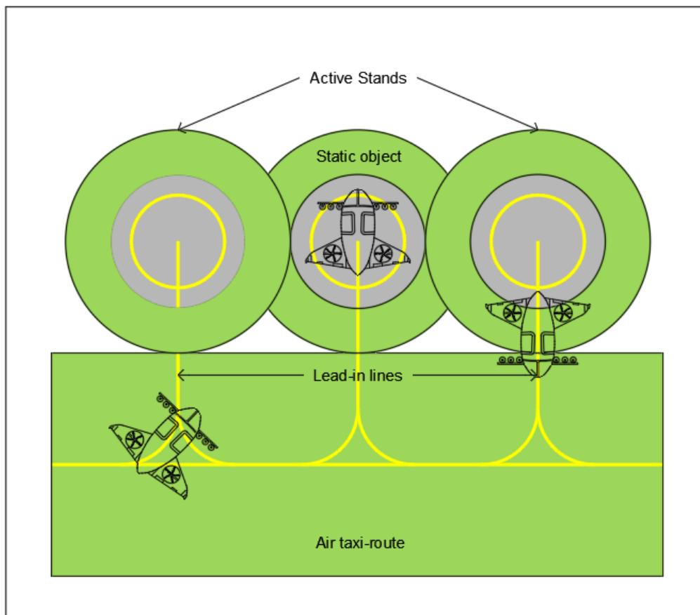
Figure C-12. Turning stands (with air taxi-routes) — non-simultaneous use — outer stands active
