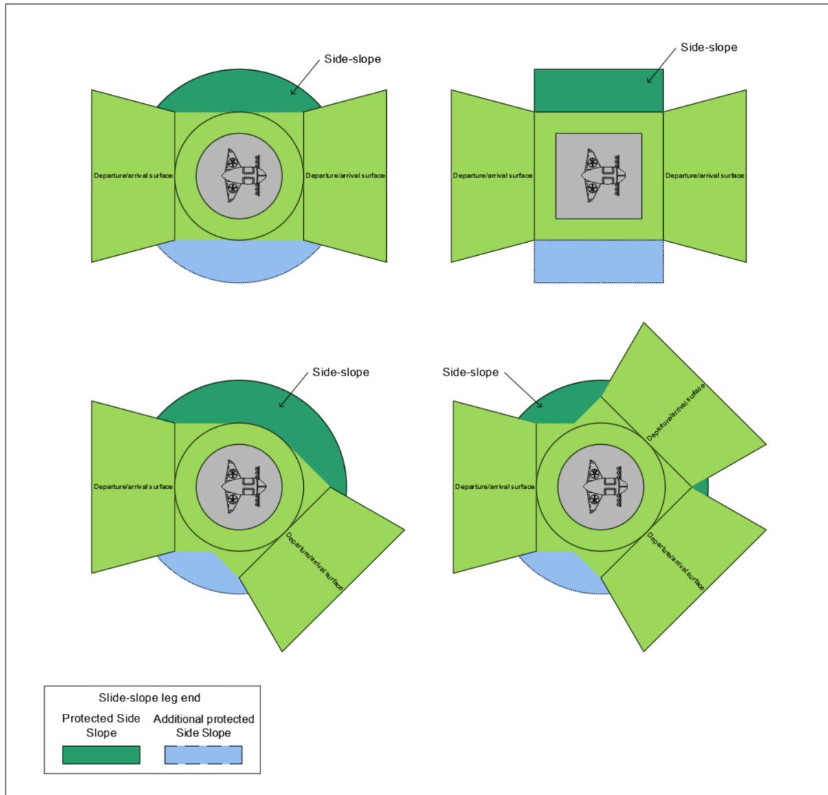
**Figure C-3.** FATO simple/complex SA and side slope protection
