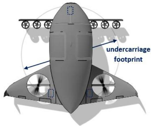
**Figure D-26.** Undercarriage footprint
