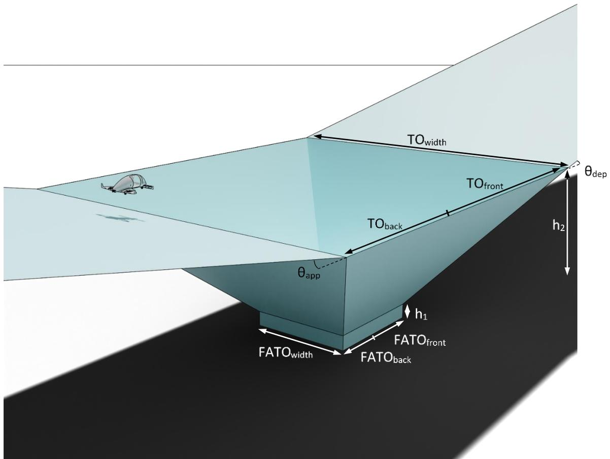
**Figure D-14.** Vertical take-off and landing procedure volume
