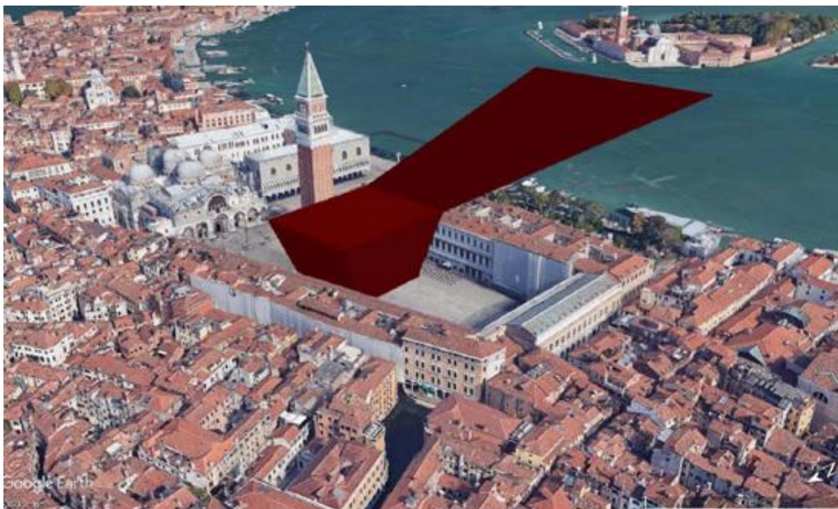
**Figure D-22.** Examples of potential vertiports with Reference volume Type 1 (for illustration purposes only; the actual suitability has not been assessed)
