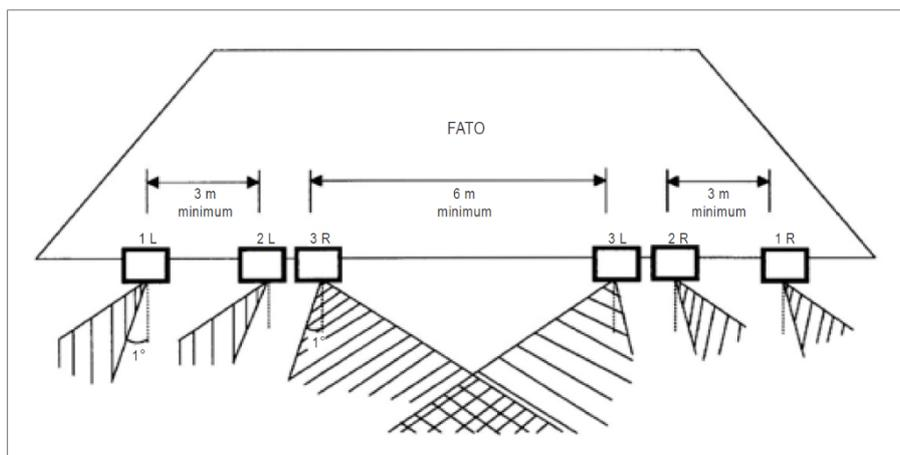
**Figure E-22.** Siting of the visual alignment guidance system
