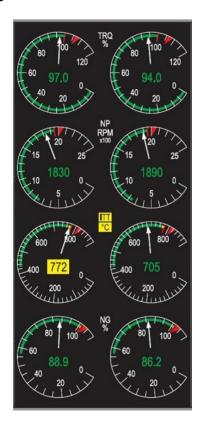
On the primary EIS indicator, where the NG are displayed in only alphanumeric format, the gas generators speed trend can be derived from analog torque indicators and ITT indicators
