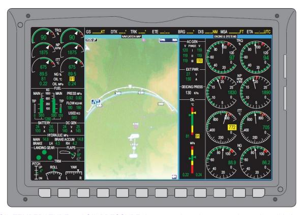
OIL TEMPERATURE and OIL PRESSURE do not require to be constantly monitored during normal operations (except engine start-up) and, contrary to TQ and ITT, they are not supposed to change rapidly. Therefore it is not essential to assess a dynamic trend, but it is necessary to be aware of the proximity of a limit value.
