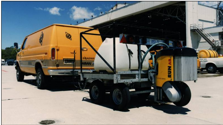
Figure 2.5: The RUNAR Variable Slip Friction Testing Device
