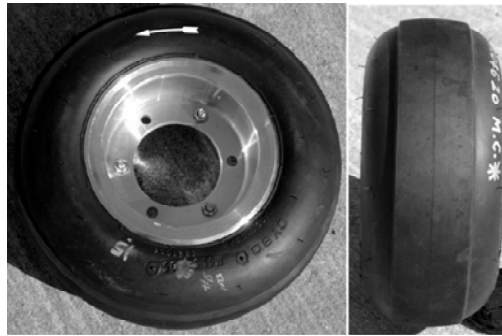
Figure 3.4: Standardized Friction Tires for the Grip Tester
