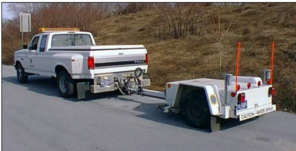
Figure 2.1: ASTM E274 Locked Wheel Testing Device
