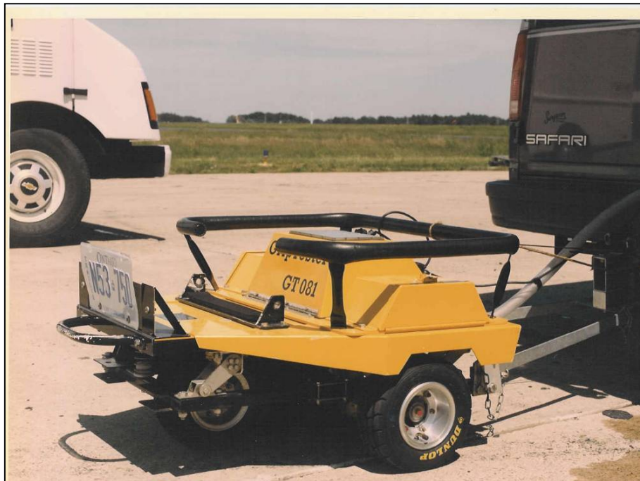
Figure 2.2: GripTester Fixed-Slip Friction Testing Device
