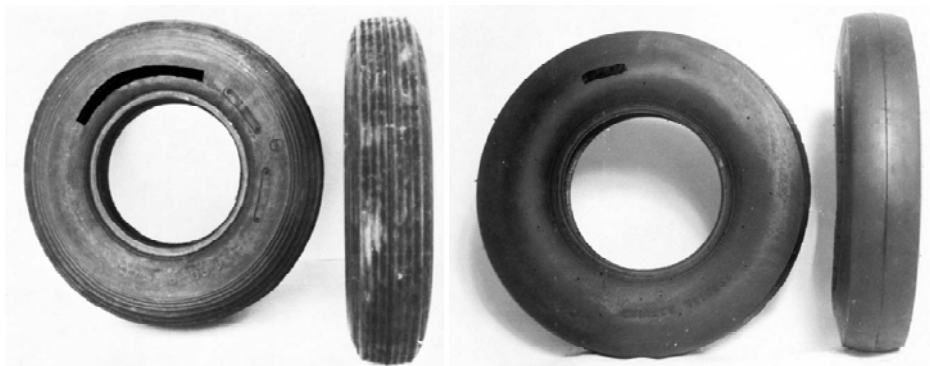
Figure 3.7: Standardized Friction Tires for the Mu-Meter Device
