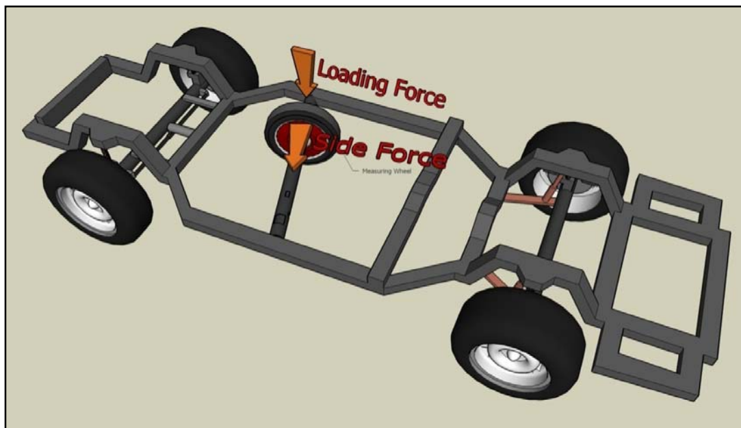
Figure 3.6: Schematic Diagram for Side Force Coefficient Measurement Principle
