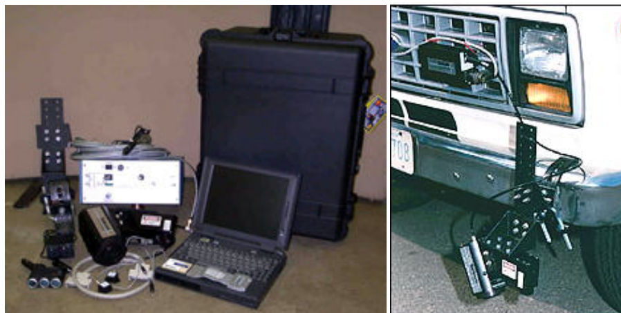
Figure 4.1: The ROad Surface Analyzer Laser Device (ROSAN).
