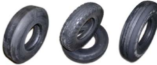
Figure 3.3: Standardized Friction Tires for SAAB, RFT, RUNAR, and other Devices
