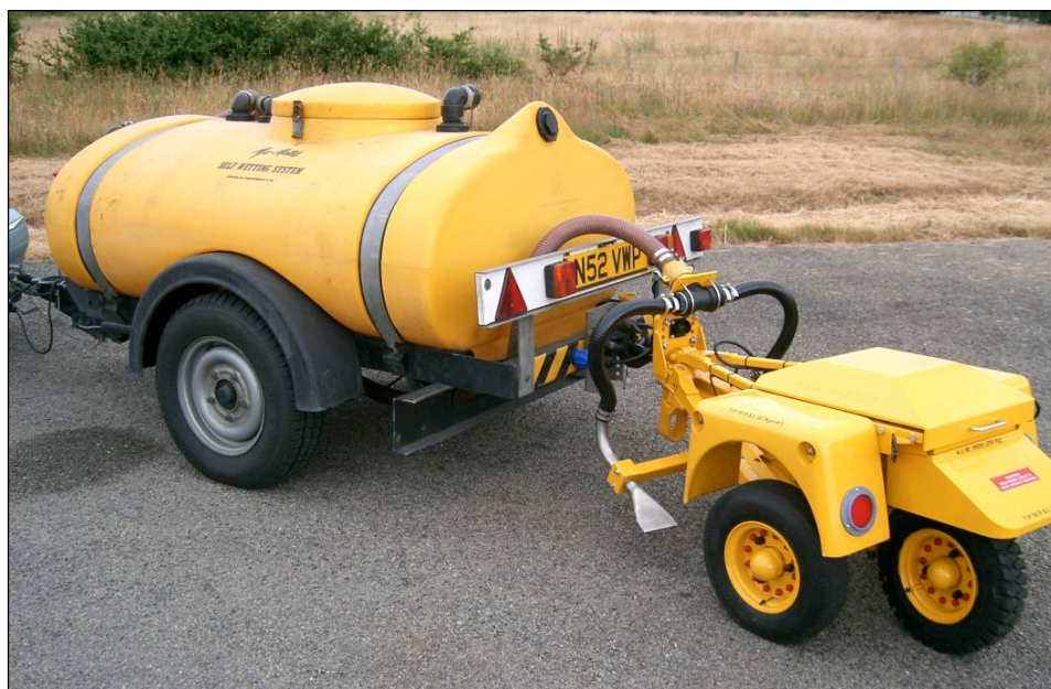
Figure 2.4: The Mu Meter Side Force Friction Testing Device
