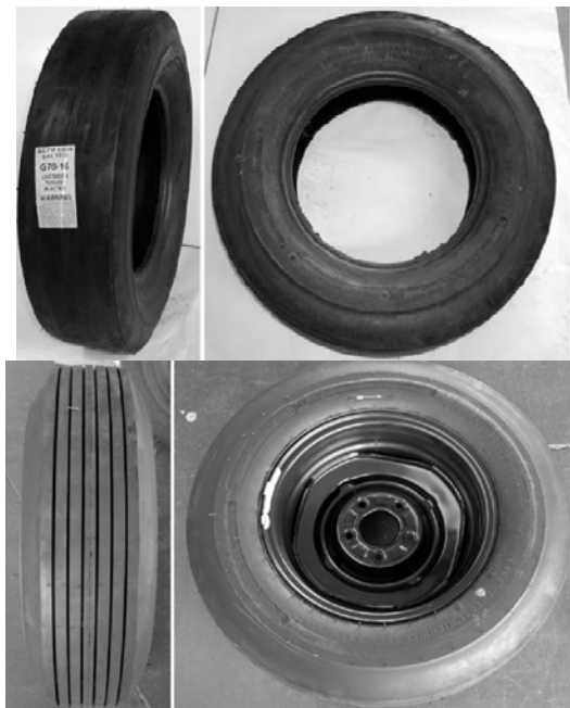
Figure 3.5: Standardized Friction Tires for the IMAG and IRV Devices
