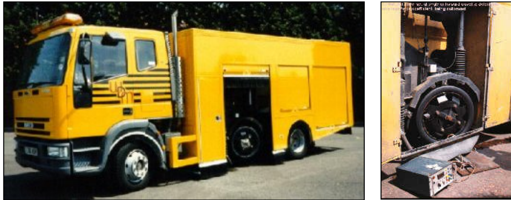
Figure 2.3: SCRIM - Sideways Force Coefficient Routine Investigation Machine
