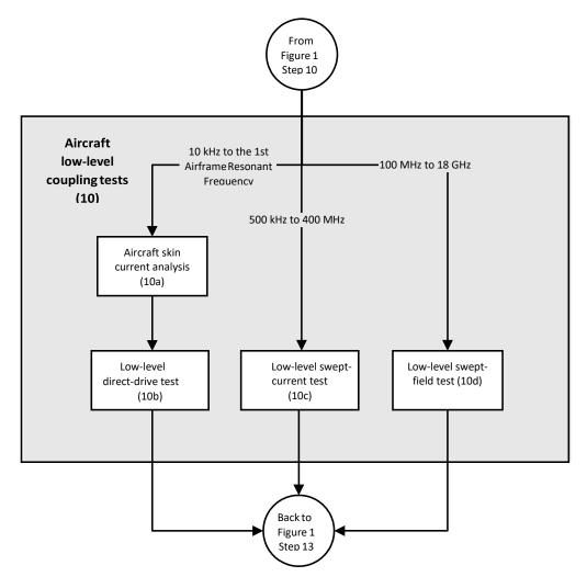
Figure 2 — Aircraft low-level coupling tests – Level A systems
