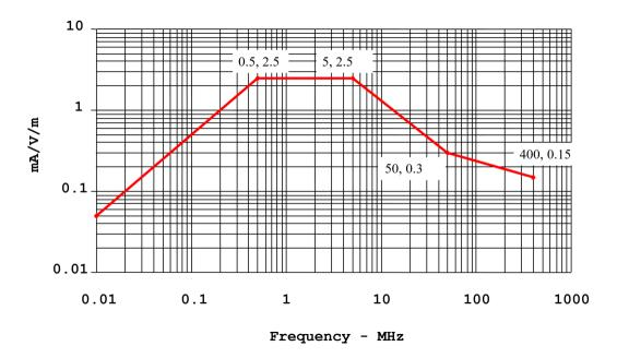
FIGURE A1-3 — Generic transfer function — Aeroplane
