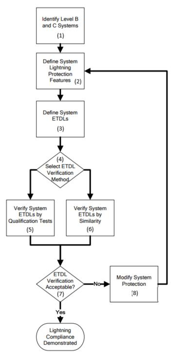
Figure 3 — Routes to lightning compliance — Level B and C systems
