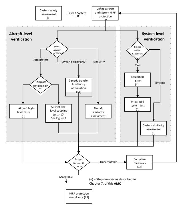
Figure 1 — Routes to HIRF compliance – Level A systems
