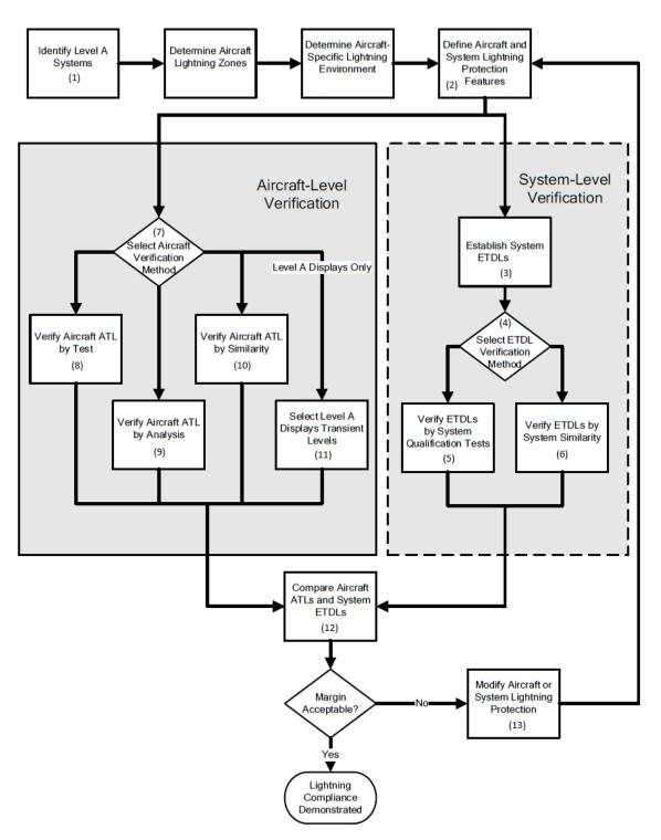
Figure 2 — Routes to lightning compliance — Level A systems
