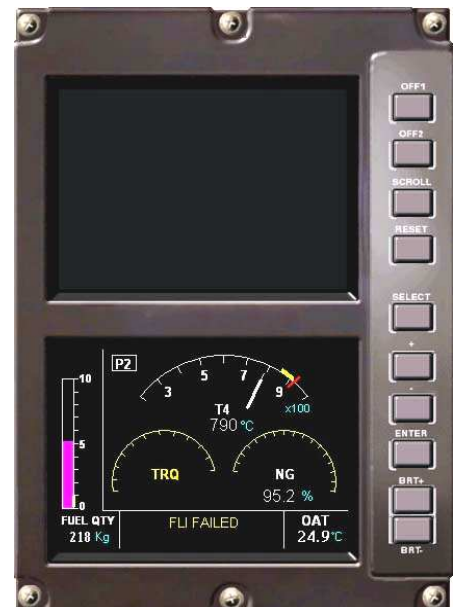
In case of upper screen information failure, remaining parameters can be read on lower screen. Here illustrated, upper screen and FLI failures.
