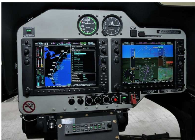
Bell 407GX / Integrated Avionics System (Garmin 1000H)
