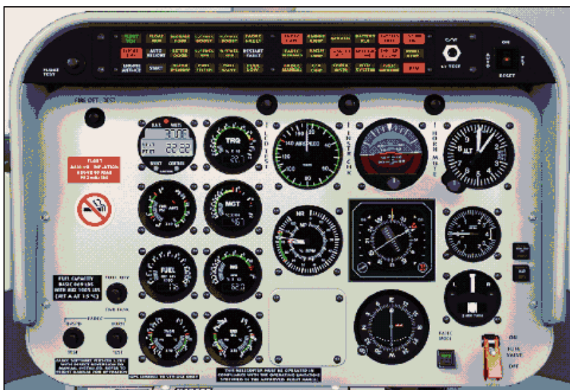
Bell 407 / Analogic Avionics
