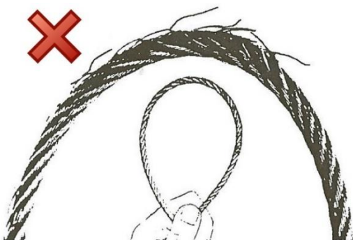
Unacceptable degradation of a control cable!
